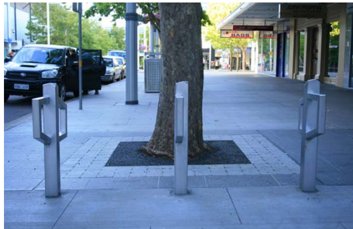
New bike railings and paving on Bunda Street
